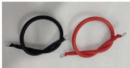
For parallel connection of battery (BLACK " - " / RED " + ")
